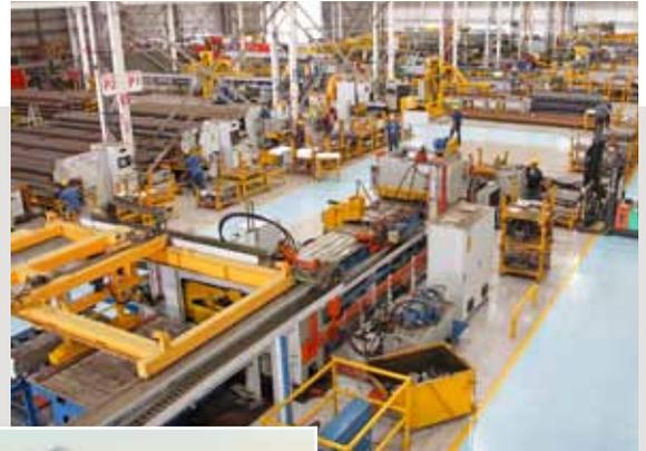
*Multiple CNC angle punch lines at Monterrey plant*
