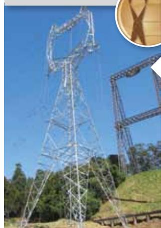
We have tested more than 600 towers at our facility in Brazil. We perform full-scale prototype testing on a wide variety of structures—accommodating heights up to 246 feet and simulating various wind, ice and snow conditions. Total transverse loads of up to 620 kips and longitudinal loads of up to 490 kips can be applied simultaneously. We now have three additional testing stations in India, including one capable of testing towers up to 1,200 kV.
